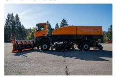
As standard, the CJS seamlessly mounts onto the Mercedes-Benz Arcos 2036 chassis type carrier vehicle. This carrier vehicle features a turning circle diameter of 18 meters and offers the option for additional rear axle steering for enhanced agility. The basic equipment and the exhaust emissions of the carrier vehicle must be selected specifically to meet the standards of the customer and the relevant country.
